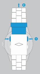
Your watch is equipped with a ratchet style wetsuit extension. This will allow you to determine the amount of extension needed with the push of a button.
