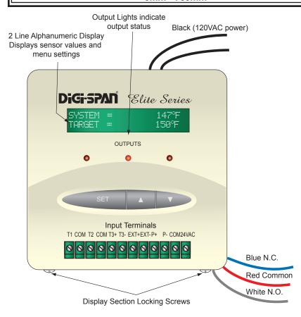
The SPC-Elite is a microprocessor based set point control that provides users with Digital Set Point capability to measure and control heating or cooling devices based on a remote temperature, pressure, vacuum, or humidity sensor Input. The Output relay is S.P.D.T thus, capable of activating or deactivating equipment and devices based on the set point and differential settings.
