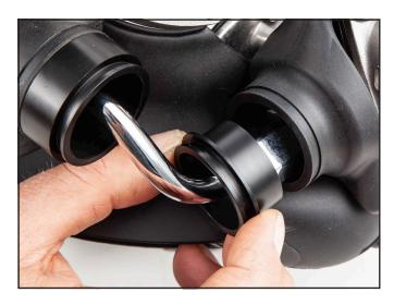
16) Line up the detail features of water tubes A & B, with the mating details of both adapter sleeves.
