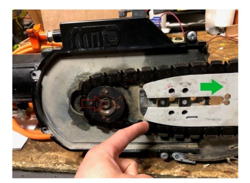
Release cover – bar becomes loose enough to slide – do not remove the cover completely Manually move the BAR outside (Green Arrow) until chain slack almost disappear – no need to tension the chain properly ( bring it out as much as you can then go back inside ¼")
