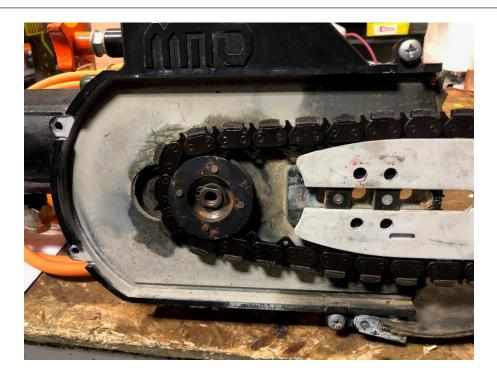
You are done! Clamp firmly the cover which is securing the bar firmly Move QT to establish desired chain tensioning You are ready to run and have an additional 1.50" of adjustment
