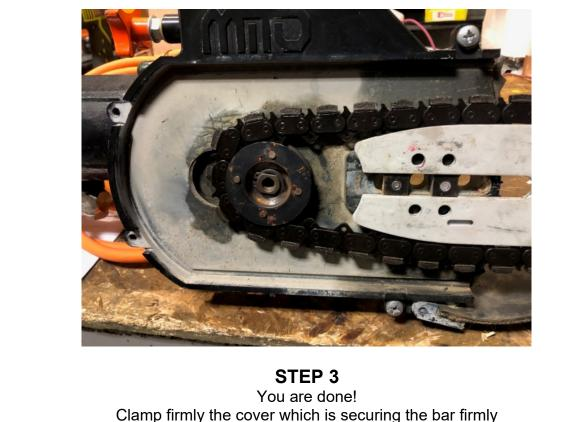
Clamp firmly the cover which is securing the bar firmly Move QT to establish desired chain tensioning You are ready to run and have an additional 1.50" of adjustment
